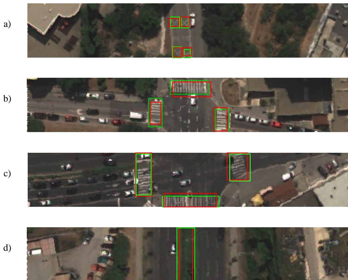
Figure 4.8 Examples of correctly detected classes by trained YOLO detector. Green bounding boxes show ground truth objects, while g boxes present predicted objects; (a) school zone markings; (b) inspected and side road pedestrian crossings, (c) inspected and side road pedestrian crossings with refuge islands as well as side pedestrian crossing on right side; (d) divided carriageways.
