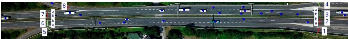
Figure 2.5 Marked characteristic locations of the observed area used for calculating location-based traffic flow parameters.
